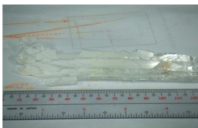
Figure 2: Quartz tube fragment showing the deposited SnO 2 nanomaterial in the inner walls
